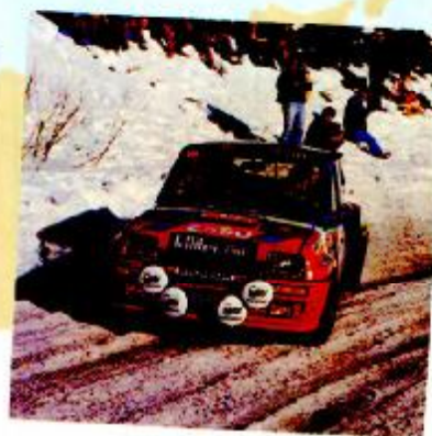
Driver Danielle Bernard Nationality French Age 31 Starting point Lisbon Car Renault 5 Gordini Engine capacity 1397 cc Maximum speed 176 km/h Petrol consumption: urban cycle 11.2 litres/100 km constant 90 km/h 6.1 litres/100 km Length 3.50 m Width 1.52 m Height 1.39 m
